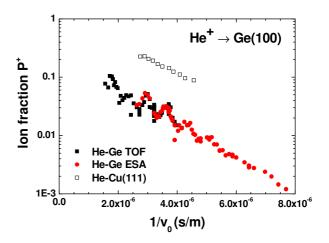
Figure 1: Ion fraction of He<sup>+</sup> scattered from a Ge(100) surface as a function of inverse initial velocity. Measurements were performed with TOF-LEIS (black) and ESA-LEIS (red) setups. P<sup>+</sup> for He<sup>+</sup>-Cu (open squares) is shown to illustrate the efficiency of qRN.
