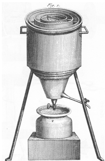
Fig. 5: Calorimeter used by Lavoisier (figure from ref. [24])
